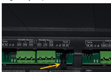
Fig. 73 Jumper inserted in only one connector
